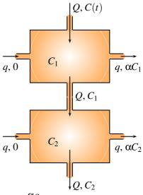
$$\begin{cases} \dot{C}_1(t) = \eta C(t) - \xi \eta C_1(t) \\ \dot{C}_2(t) = \eta C_1(t) - \xi \eta C_2(t) \end{cases} \quad \text{où } \eta = \frac{Q}{V}, \quad \xi = \frac{\alpha q}{Q}$$
